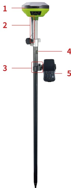
Figure 4.11 LUKA as a Rover - Internal Radio
