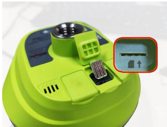
Figure 2.1 Insert the SIM card
