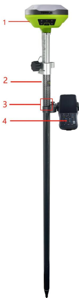
Figure 2.3 LUKA as a rover without radio antenna
