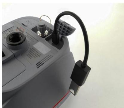
Figure7 Connect Oscar to a USB flash drive
