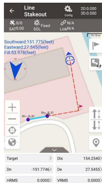
Figure 4.17 Stakeout a straight line
