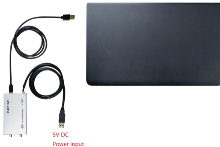
Figure 2.10 BX316D Enclosure connected to a Laptop
