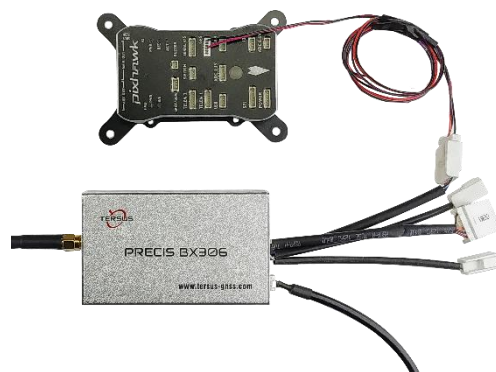
Figure 5.23 Outline of BX306 connected to Pixhawk
