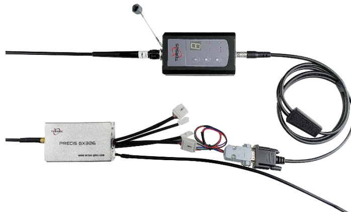
Figure 5.21 Outline of BX306 Connected to RS460 Radio
