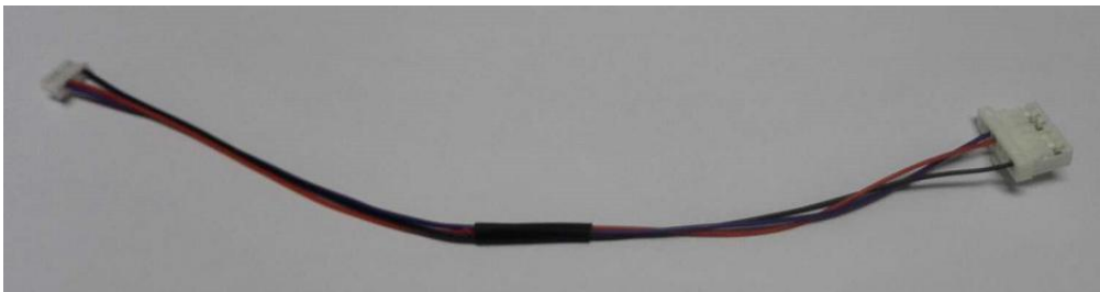
Figure 5.22 Cable between Pixhawk and BX306
