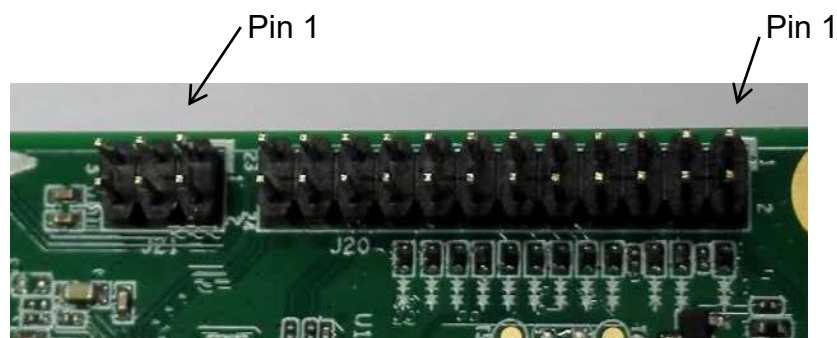
Figure 4.6 Connectors J20 and J21 of BX306Z
