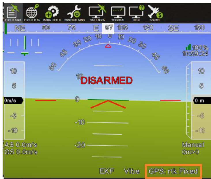
Figure 5.26 GPS status changes to rtk Fixed
