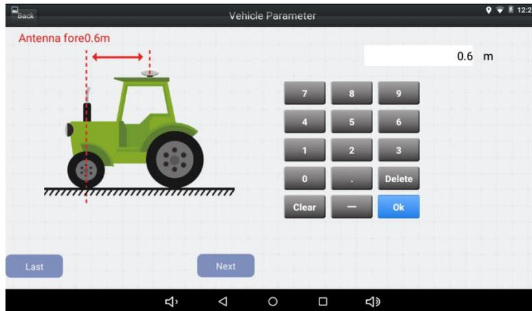
Figure 2.33 Vehicle parameter configuration – antenna fore
