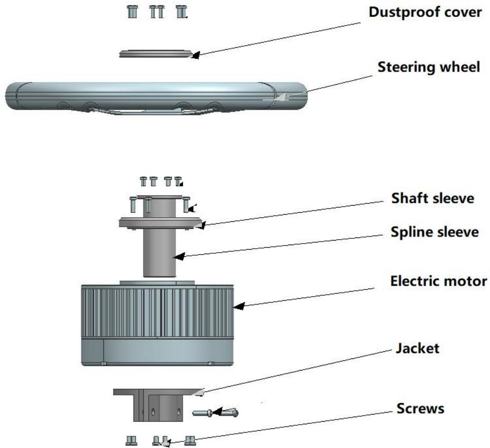
Figure 2.2 Descriptions of the EMS2 assembly components
