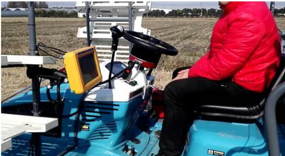
Figure 4.3 Transplanting using AG990 auto-steering system
