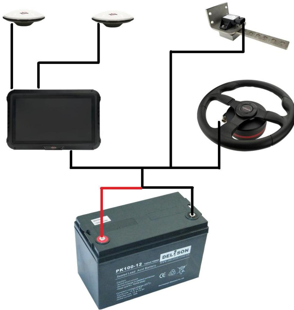
Figure 1.2 AG990 auto-steering system structure
