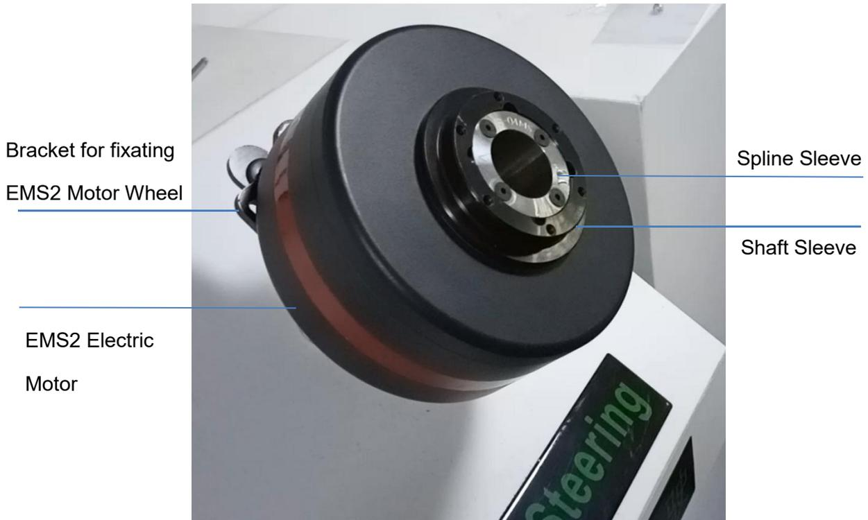
Figure 2.4 Installation example of electric motor
