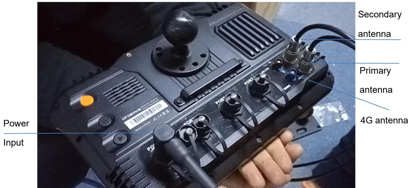
Figure 2.23 T100 Control Tablet connects to main cable and two antennas
