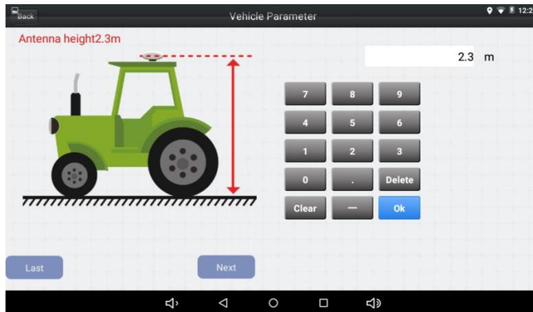
Figure 2.30 Vehicle parameter configuration – antenna height
