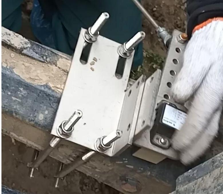
Figure 2.9 Possible position of angle sensor – 1
