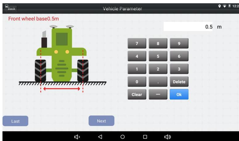
Figure 2.35 Vehicle parameter configuration – front wheel
