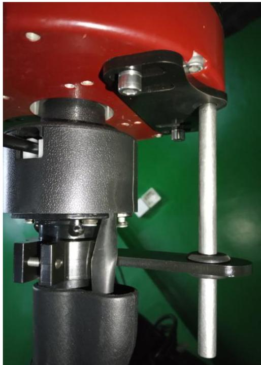
Figure 2.5 Installation example of bracket for fixating EMS2 Motor Wheel
