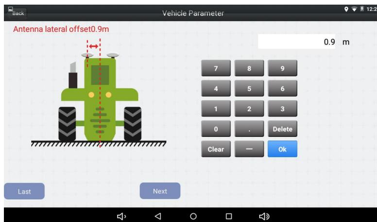
Figure 2.31 Vehicle parameter configuration – antenna lateral offset
