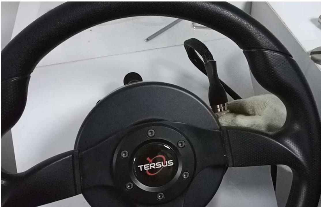
Figure 2.22 Main Cable connects to EMS2 Motor Wheel
