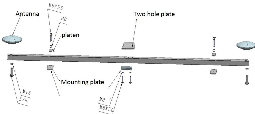
Figure 2.13 Descriptions of dual-antenna components
