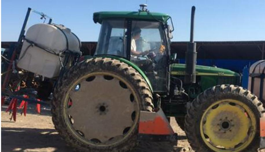
Figure 4.2 Spraying pesticide using AG990 auto-steering system
