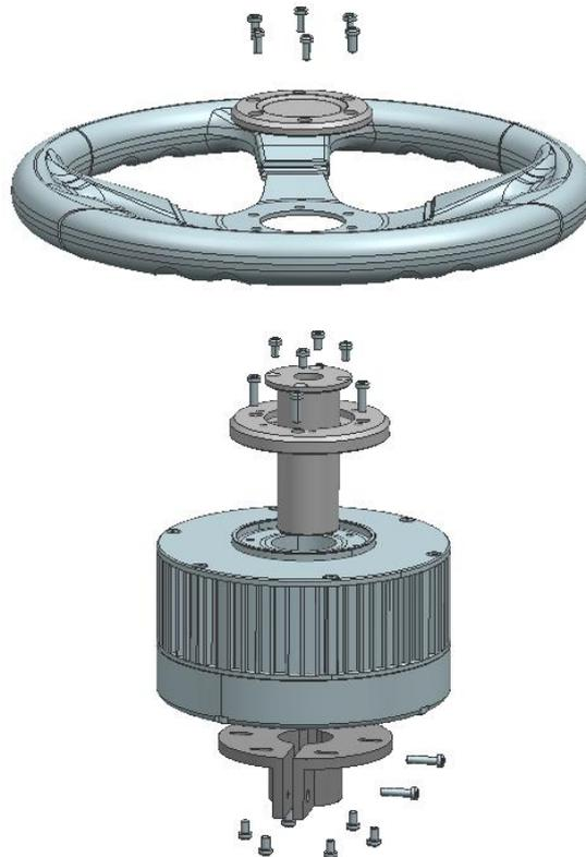
Figure 2.1 Assembly diagram of EMS2 motor wheel
