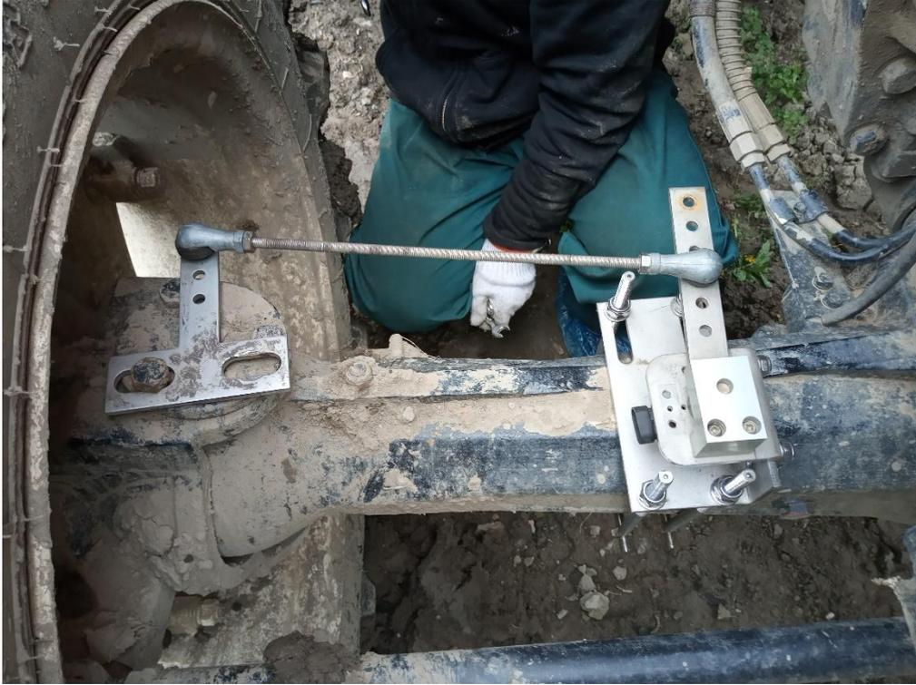
Figure 2.11 Installation example of angle sensor
