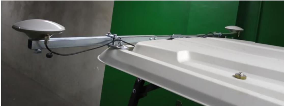
Figure 2.15 Installation example of dual-antenna – 2
