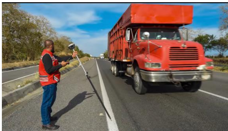
Figure 5.1 Tilt survey– on the high way
