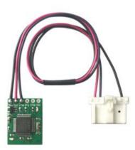
Figure 5.14 Data logger DL207
