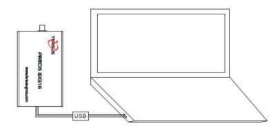
Figure 5.2 Download Files from eMMC Card with an USB Port
