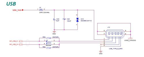
Figure 4.5 Reference Schematic for USB
