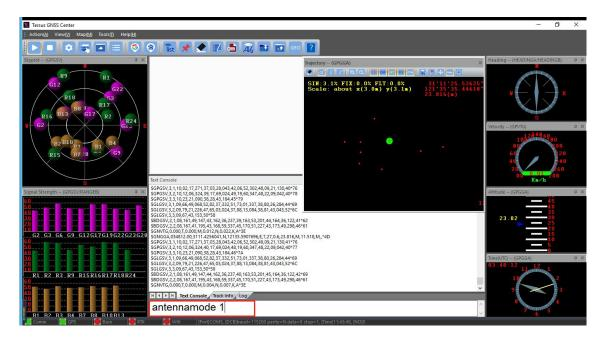
Figure 2.24 Set antenna mode to GPS & GLONASS
