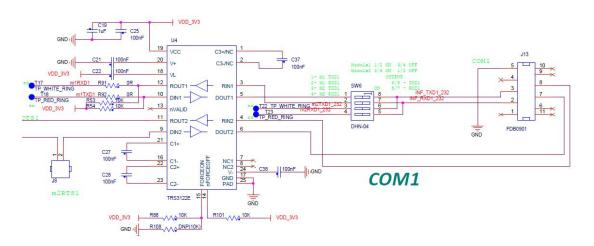
Figure 4.4 Reference Schematic for a Serial Port
