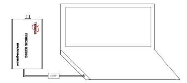
Figure 5.1 Download Files from eMMC Card with a Serial Port
