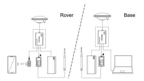
Figure 2.14 Base/Rover Configure
