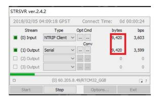
Figure 5.19 Input and Output data in progress
