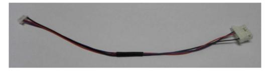
Figure 5.22 Cable between Pixhawk and BX306
