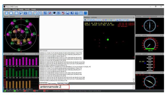
Figure 2.25 Set antenna mode to GPS & BeiDou
