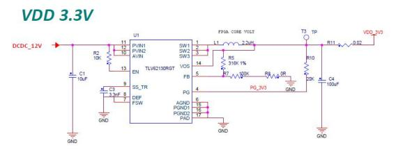
Figure 4.2 3.3V Reference Schematic
