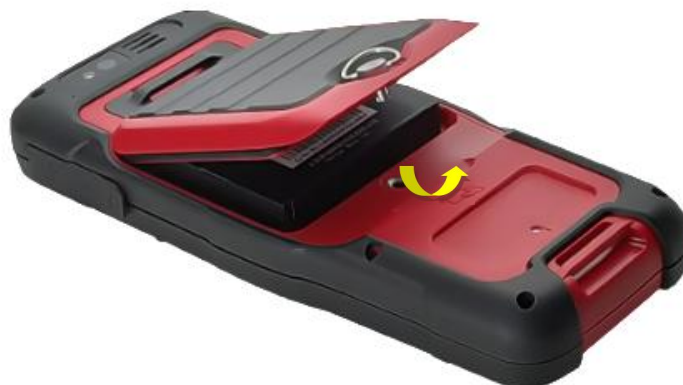
Figure 2.19 Take off the back cover
