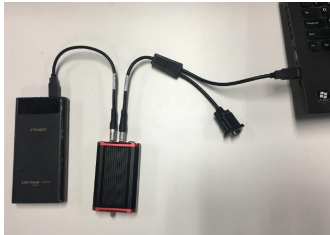
Figure 7.2 Connections of David, computer and power bank
