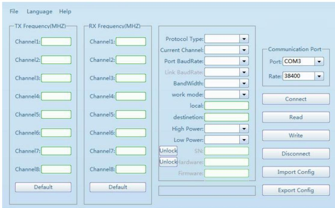
Figure 3 Interface of configuration tool
