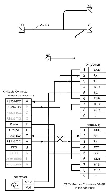
Fig.5.9. The diagram of the interface cable 2 for the Tersus INS connections to two COM-ports of the host computer and to the AC/DC adapter
