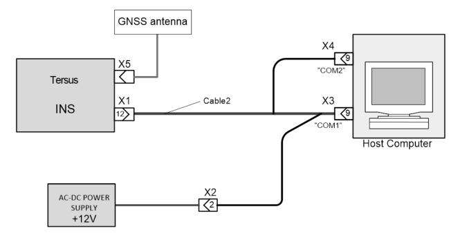
Fig.5.6. The diagram of electric connection of the Tersus INS to PC with output of the raw GNSS data or NMEA data set
