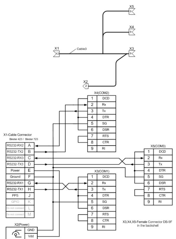
Fig.5.10. The diagram of the interface cable 3 for the Tersus INS connections to two COM-ports of the host computer, to radio modem and to the AC/DC adapter
