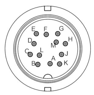
Fig.5.3. The Tersus INS RS-232 connector pinout (mating side of the connector)
