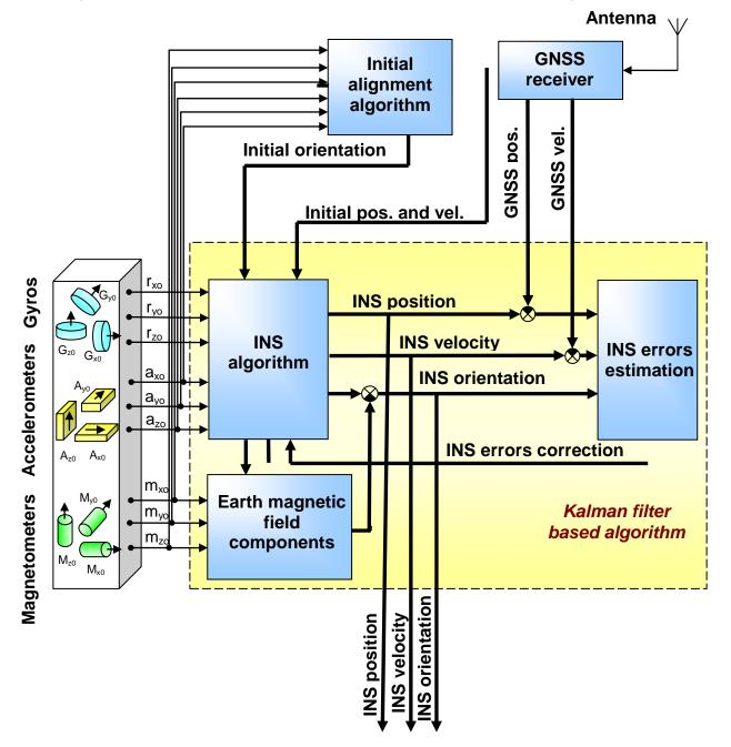
Fig.2.1. Operational Diagram of the Tersus INS
