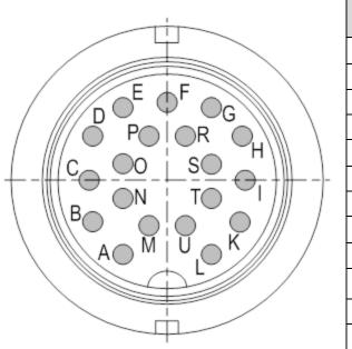
Fig.5.4. The Tersus INS RS-422 connector pinout (mating side of the connector)
