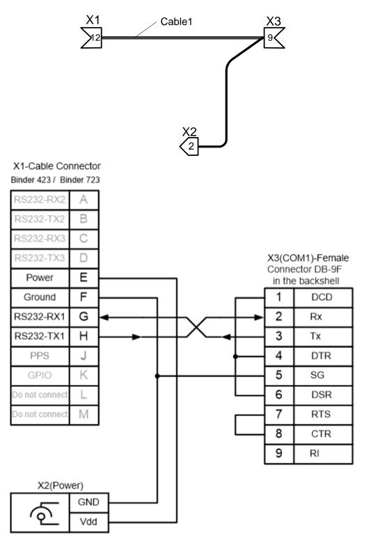
Fig.5.8. The diagram of the interface cable 1 for the Tersus INS connection to the COM-port of the host computer and to the AC/DC adapter
