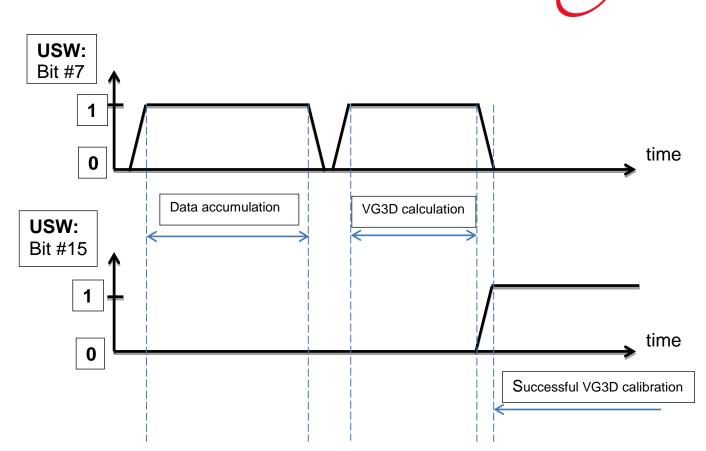
Fig.6.1. The diagram of indication of on-the-fly VG3D calibration procedure in the USW (Unit Status Word, see section 6.9)
