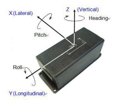
Fig.1.3. Coordinate system of the Tersus INS
