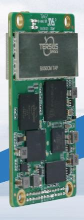
**GNSS OEM Boards & Module**
