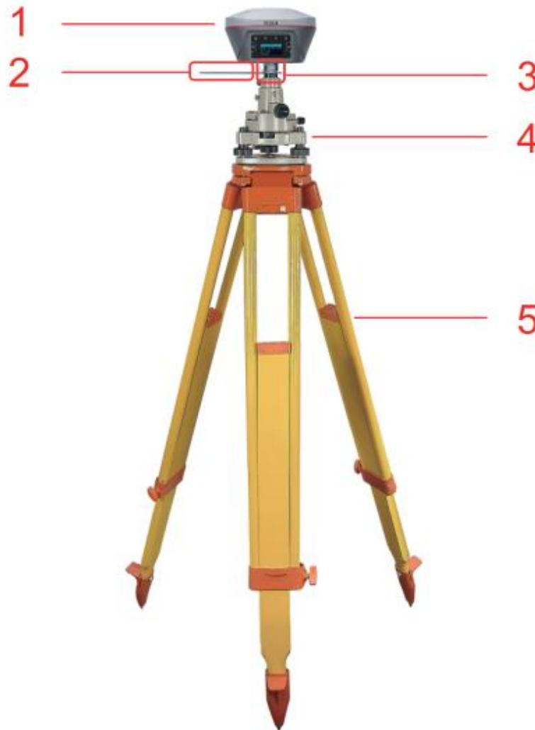
Figure 2.4 Oscar as a base without radio antenna
