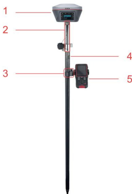
Figure 4.11 Oscar as a Rover - Internal Radio
