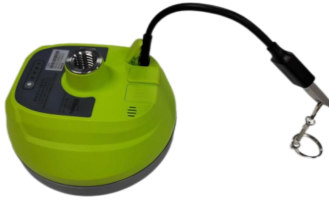
Figure 5 Connect LUKA to a USB flash drive
