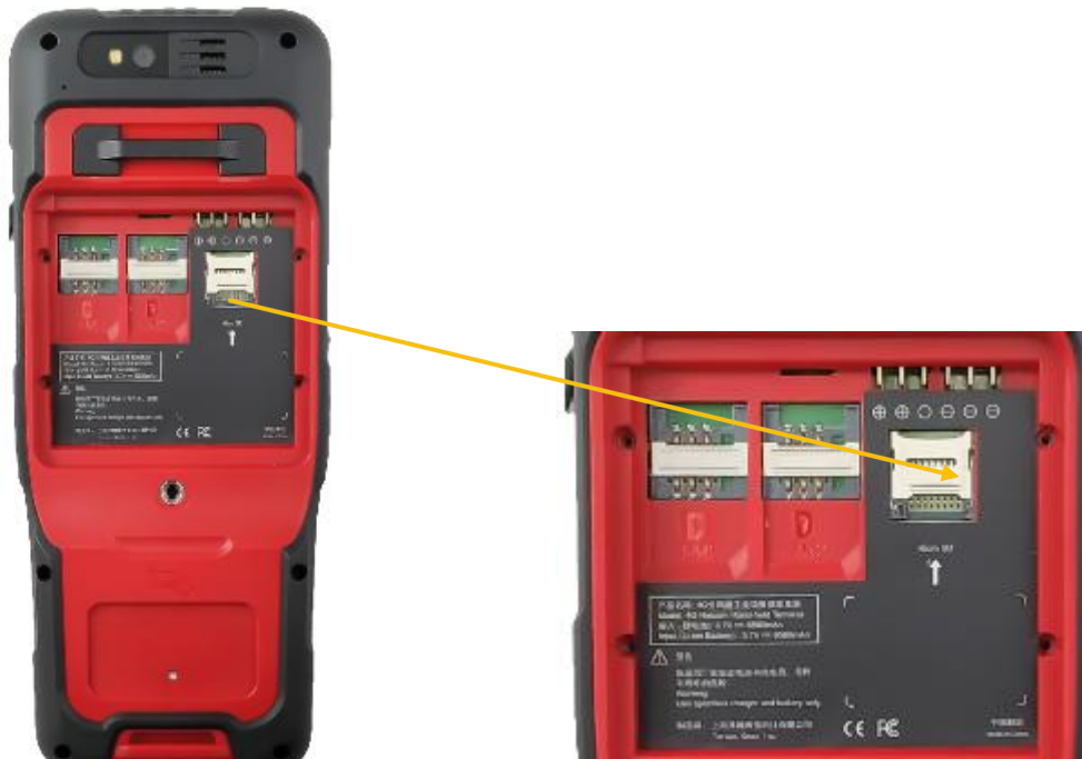
Figure 6.11 Insert Micro SD card
