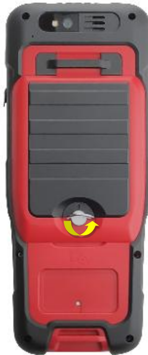
Figure 6.8 Remove the back cover
