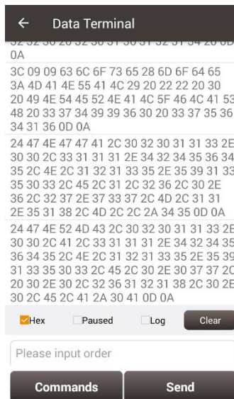
Figure 3.16 Data Terminal outputs hex data
