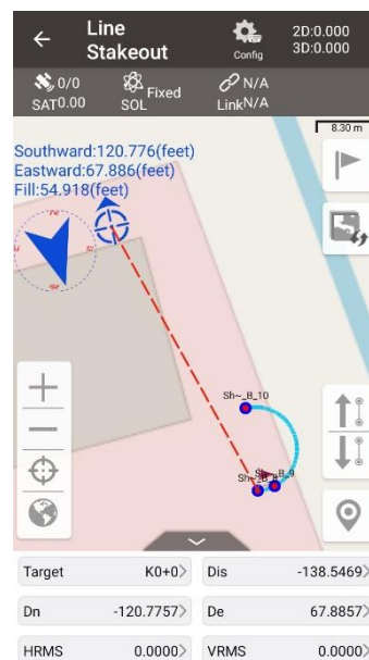
Figure 4.21 Stakeout an arc
