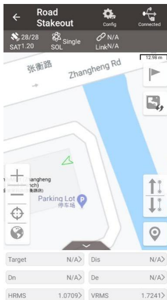
Figure 4.65 Road stakeout interface
