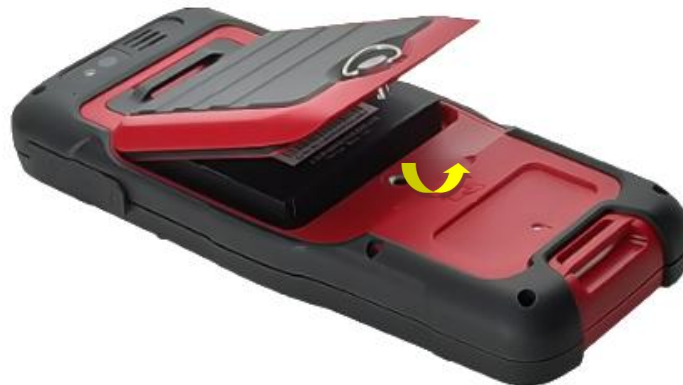
Figure 6.8 Take off the back cover
