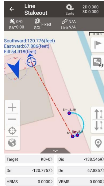
Figure 4.23 Stakeout an arc
