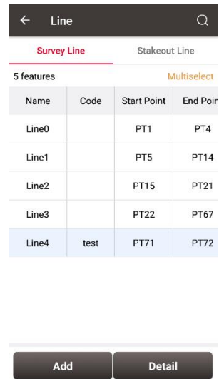
Figure 2.77 Survey line interface
