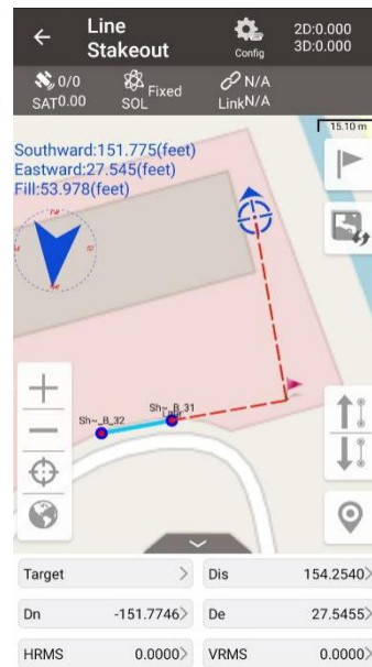
Figure 4.19 Stakeout a straight line
