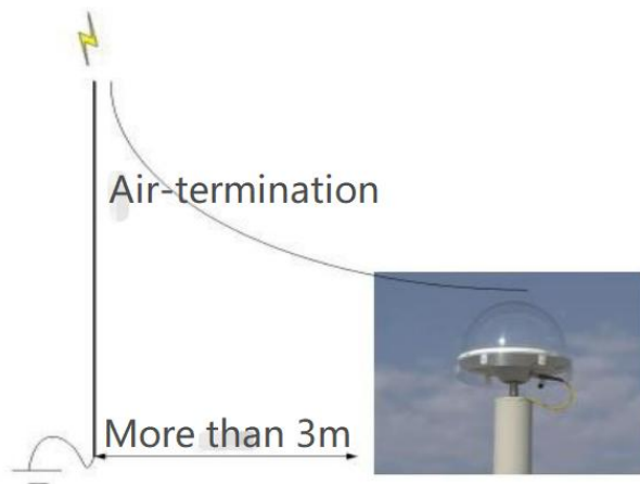
Figure 5.1 Schematic diagram of direct lightning prevention
