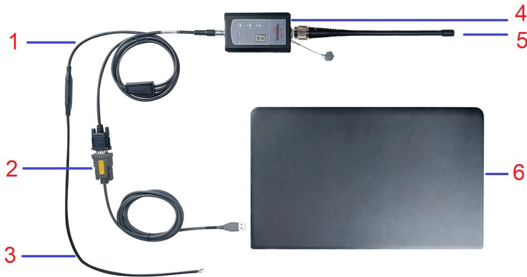
Figure 2.2 Hardware connection for software configuration
