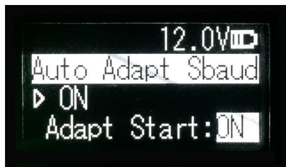
Figure 2.7 Serial baud rate self-adaption
