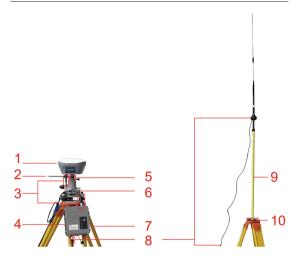
Figure 1.3 Oscar as a Base – External Radio RS400H2
